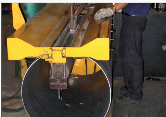
Longitudinal Joint Welding
